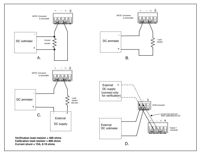
Figure B-1. Verification and Calibration Test Setup
